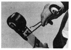
Make sure that the roller ski is well-supported. Place the ends of support strut vertically on slots in fork plates.
